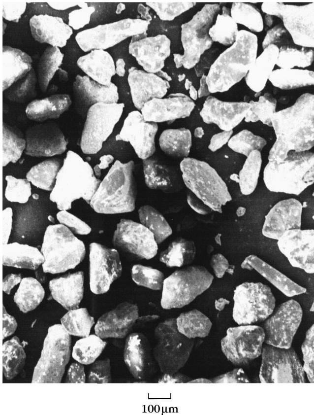
FIG. 1. Scanning electron micrography of quartz sand sediment particles.
